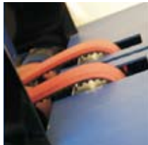
Sliding levers upward raises the elevator belts to increase friction
