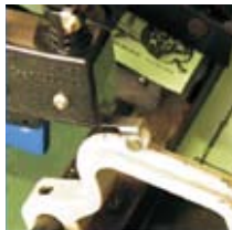
Hold down arm activates feeder
