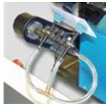
The reciprocating Arm grabs the product with two suction cups
