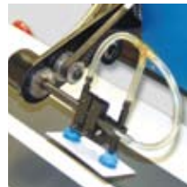
Once the Pick Arm makes its full 180 degree turn, it places the product directly where you want it
